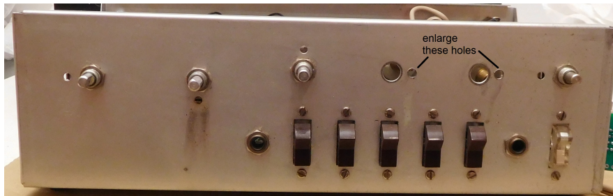
Figure 6-Enlarge the locator tab holes for bass and treble controls
