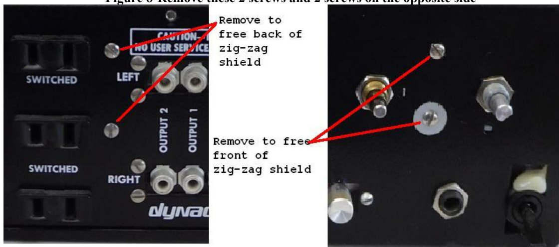
Figure 9-Remove the screws and nuts that hold the zig-zag shield to back and front of chassis
