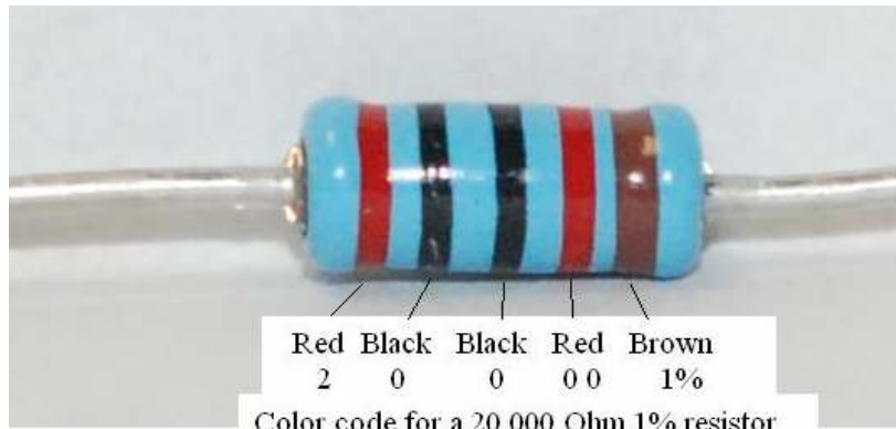
Figure 18-demonstrating the resistor color code
