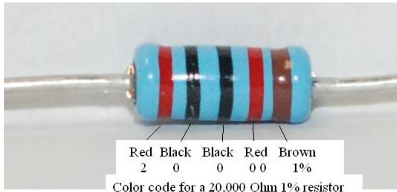
Figure 11-demonstrating the resistor color code
