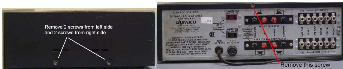
Figure 1-Side and Back views showing location of cover retaining screws
