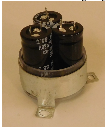
Figure 2-Triple cap installed into the capacitor clamp
