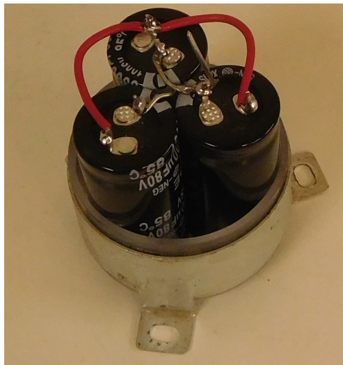
Figure 4-Soldering the ground and positive harnesses on the new C9 dynamite capacitor arrangement
