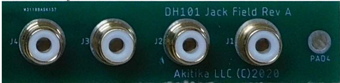
Figure 1-Insert the jacks into the silk-screen side
