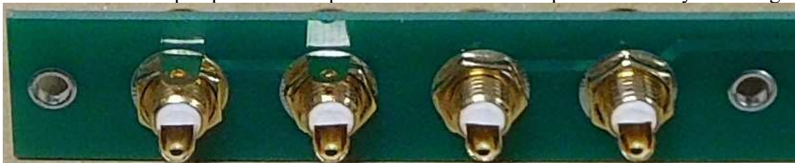
Figure 3-orientation of lugs and solder cups
