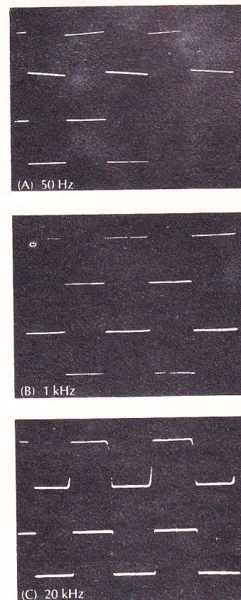
Fig. 2—Oscilloscope traces of PAT-4 square-wave response.
