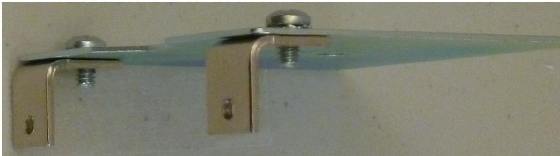
Figure 3-Fastening brackets to mounting plate
