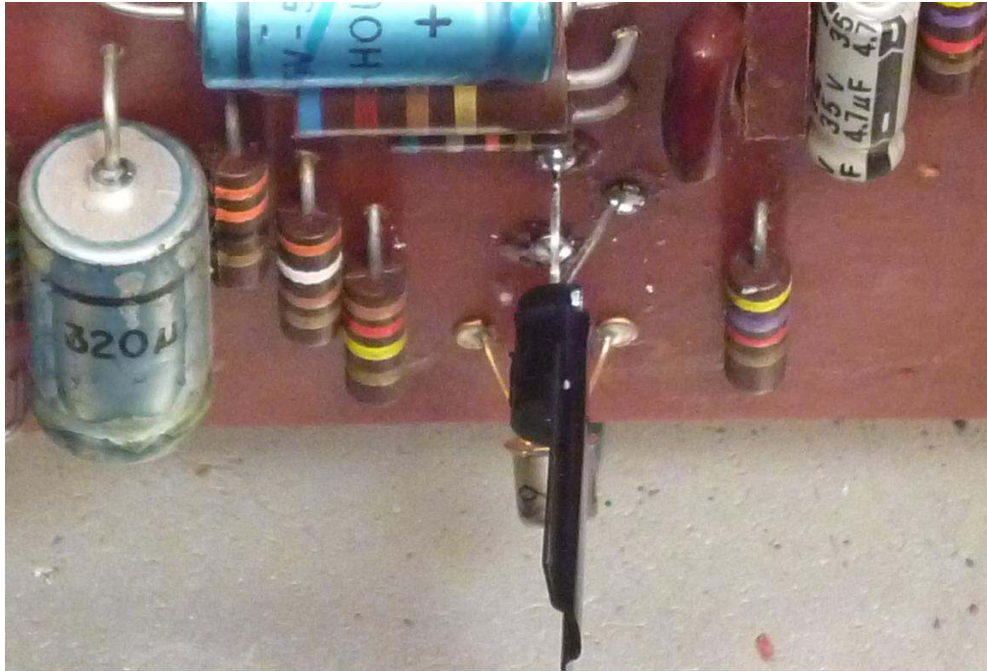
Figure 2-New transistor with heatsink installed on PCB
