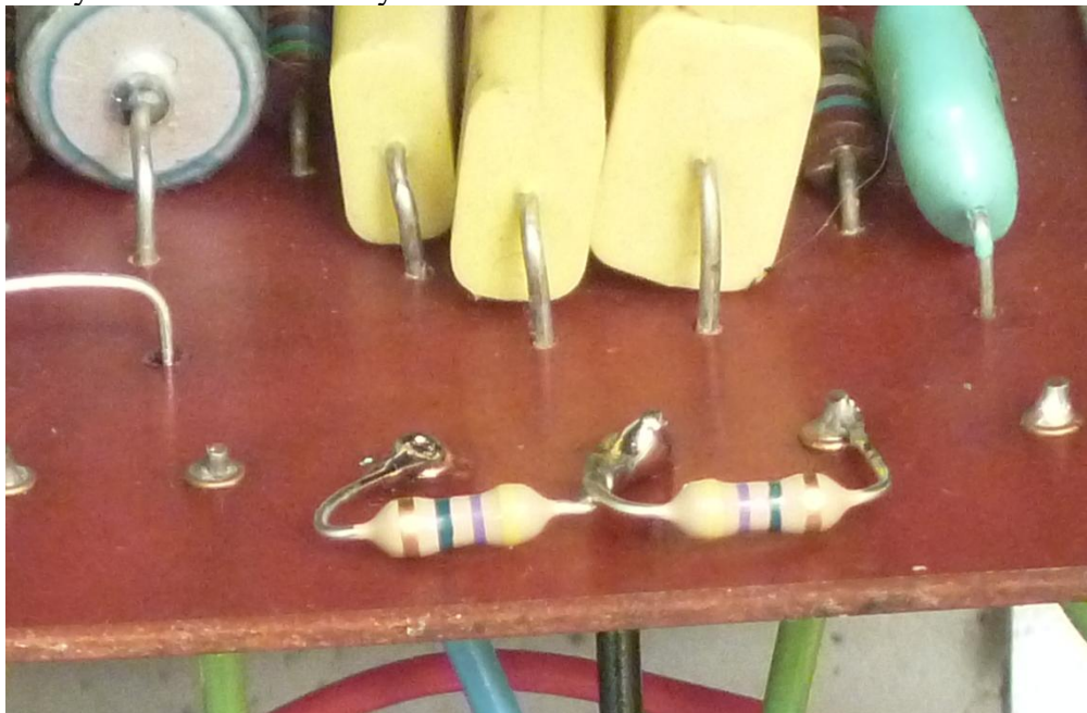
Figure 7-Installing the treble no-click resistors on eyelets 16, 17, and 18
