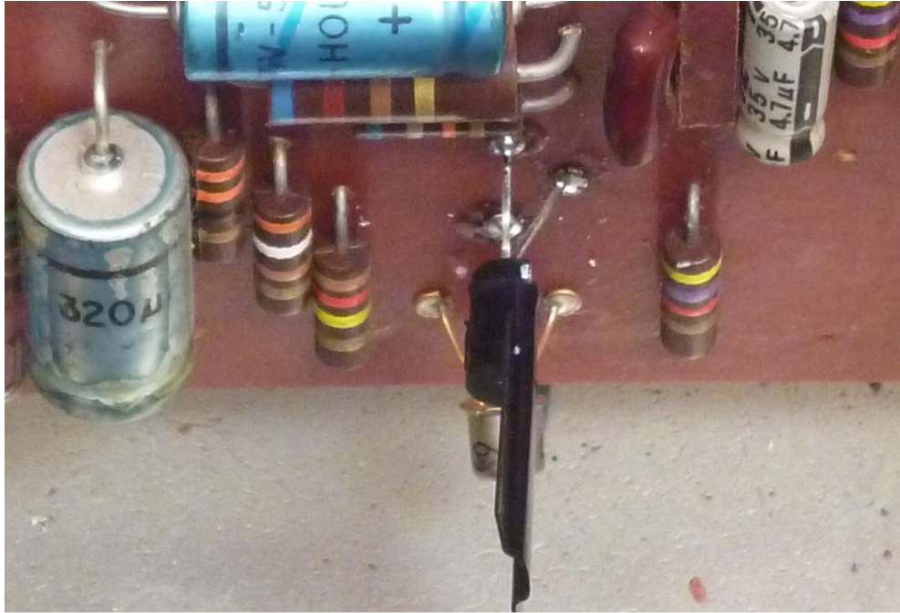
Figure 3-New transistor with heatsink installed on PCB
