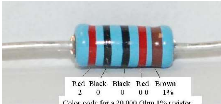
Figure 18-demonstrating the resistor color code
