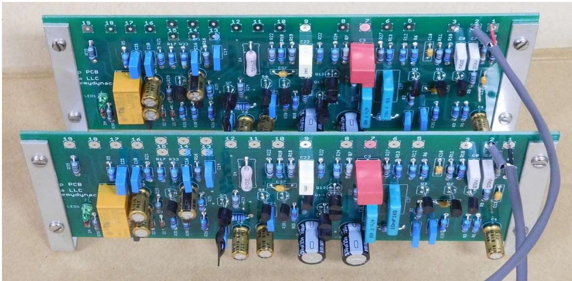
Figure 13-Re-use the original 4-40 screws to re-attach mounting brackets to the PCBs
