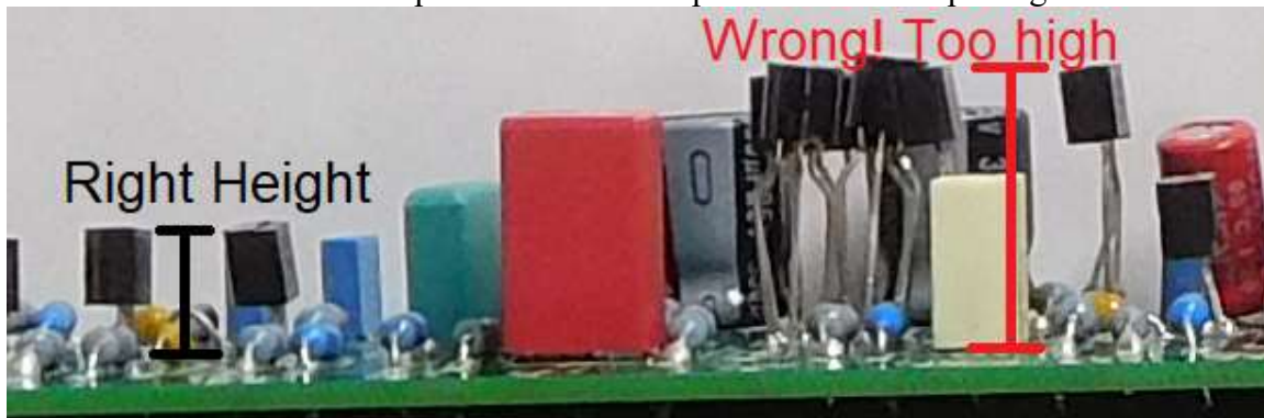
Figure 6-Proper height for transistor installation
