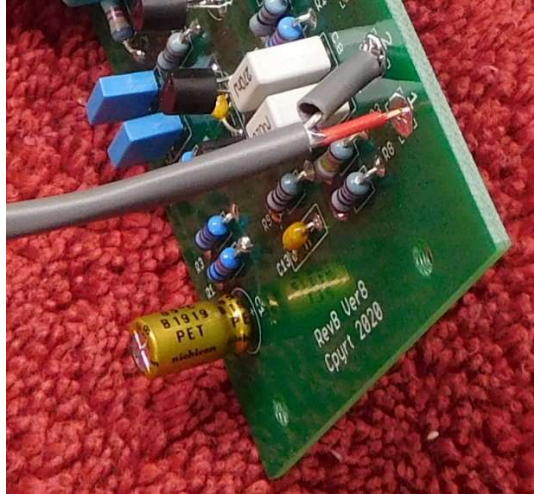
Figure 8-Shielded cable installation (right channel shown here)
