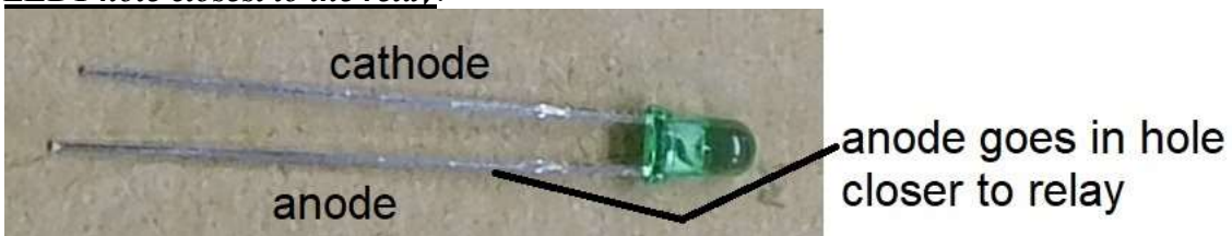
Figure 7-Closeup of LED, note anode is longer
