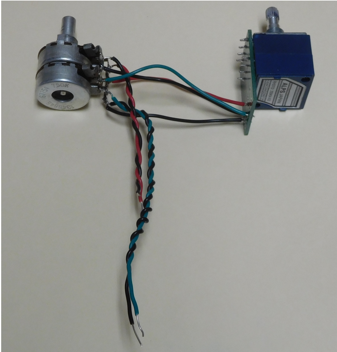
Figure 10-completed balance-volume assembly ready for installation
