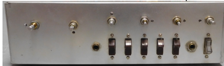
Figure 4-Viewing the structural front panel with the cosmetic front panel removed
