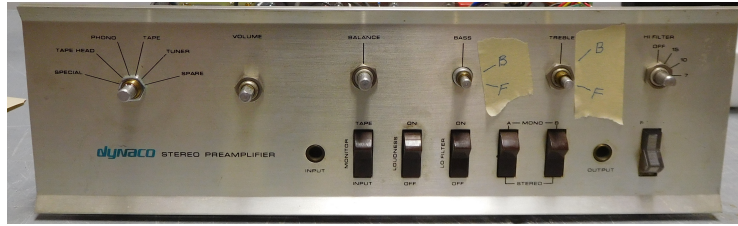
Figure 3-knobs removed, note markings for clockwise positions of tone controls
