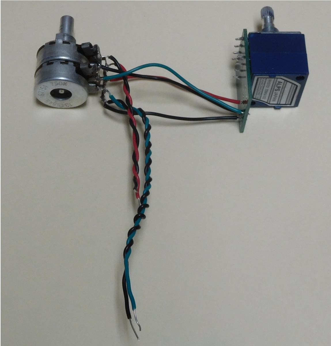
Figure 7-completed balance-volume assembly ready for installation
