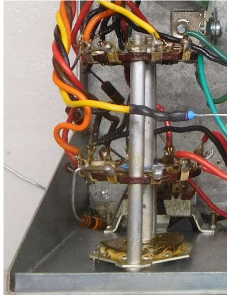
Figure 7-Resistor, wire, and heat-shrink tubing
