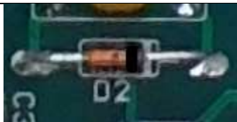
Figure 3-match black band on diode to white stripe on PCB
