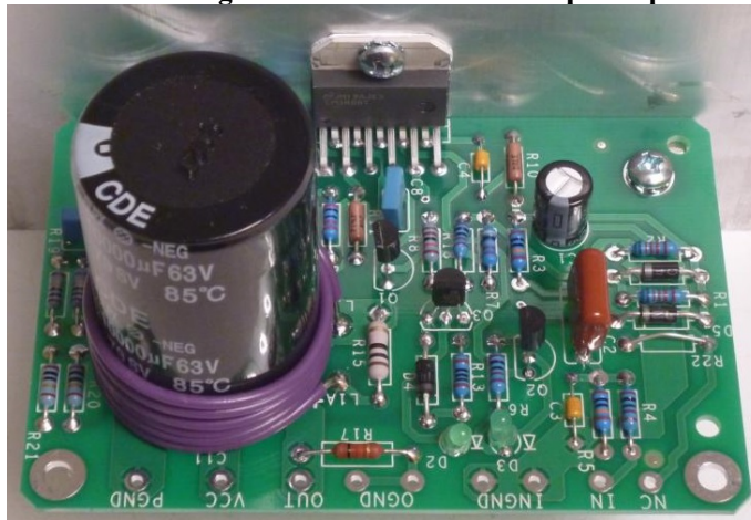
Figure 25-The LM3886 sits up off the board to avoid shorts between the front and back rows of pins. The body should be at right angles to the circuit board
