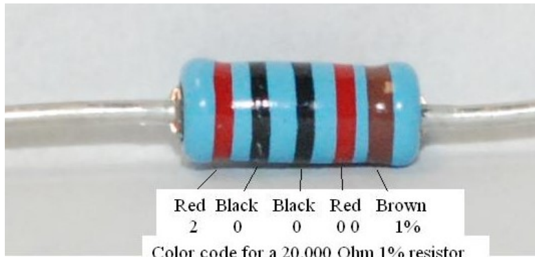
Figure 32-demonstrating the resistor color code
