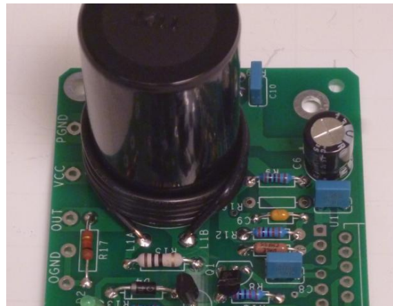
Figure 23-finishing step for the output inductor
