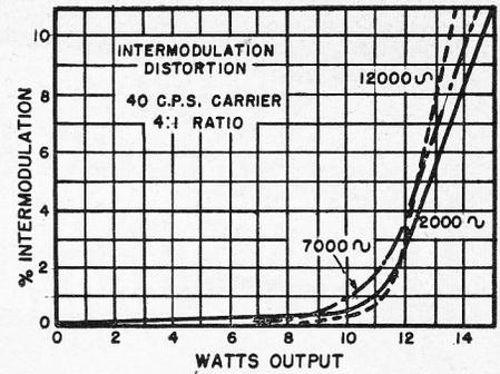
Fig. 4. Intermodulation distortion.
