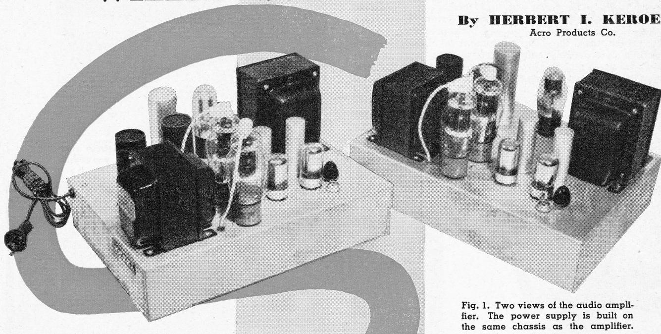
Fig. 1. Two views of the audio amplifier. The power supply is built on the same chassis as the amplifier.
