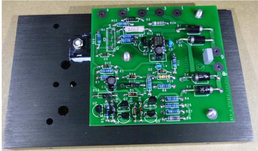
Figure 10—installing the PC board on the heat sink
