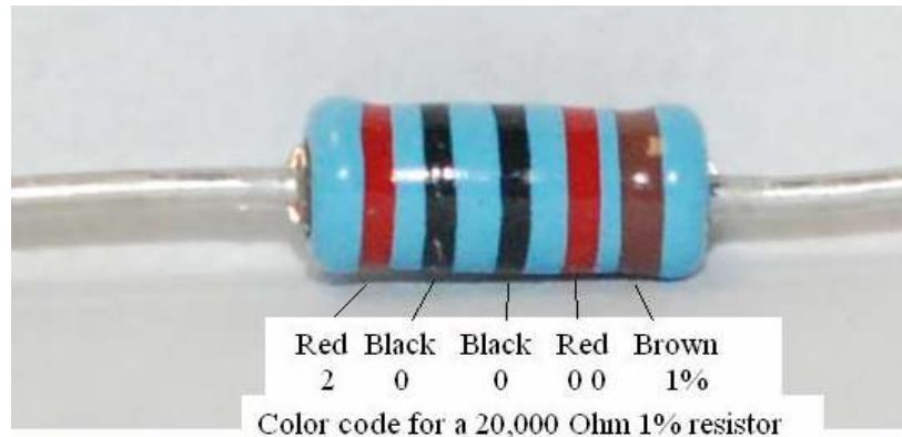
Figure 16-demonstrating the resistor color code
