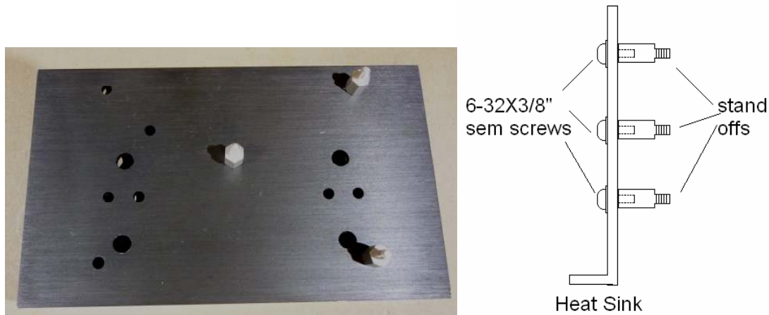
Figure 6-Installing the stand-offs. Picture on left shows location, picture on right shows side view of assembly detail
