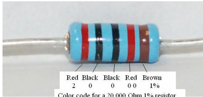
Figure 24-demonstrating the resistor color code
