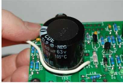
Figure 12-Starting to wind the output inductor
