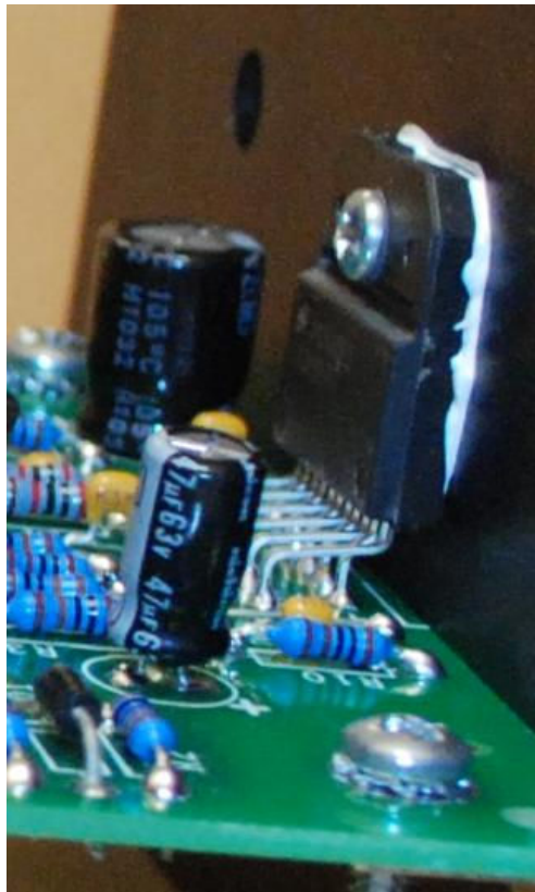
Figure 17-The LM3886 sits up off the board to avoid shorts between the front and back rows of pins. The body should be at right angles to the circuit board
