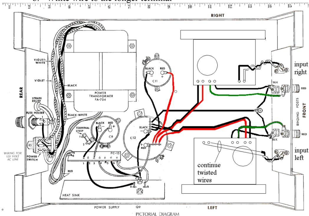
Figure 19-completed wiring
