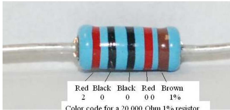
Figure 22-demonstrating the resistor color code
