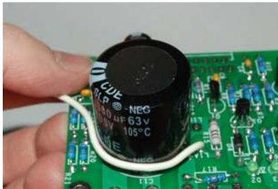
Figure 12-Starting to wind the output inductor
