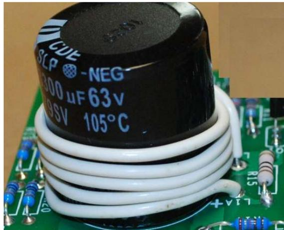
Figure 13-finishing step for the output inductor
