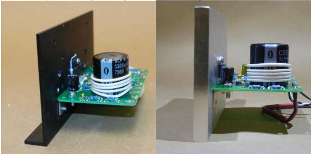
**Figure 17-completed amplifier moduled on original and super heatsinks**
