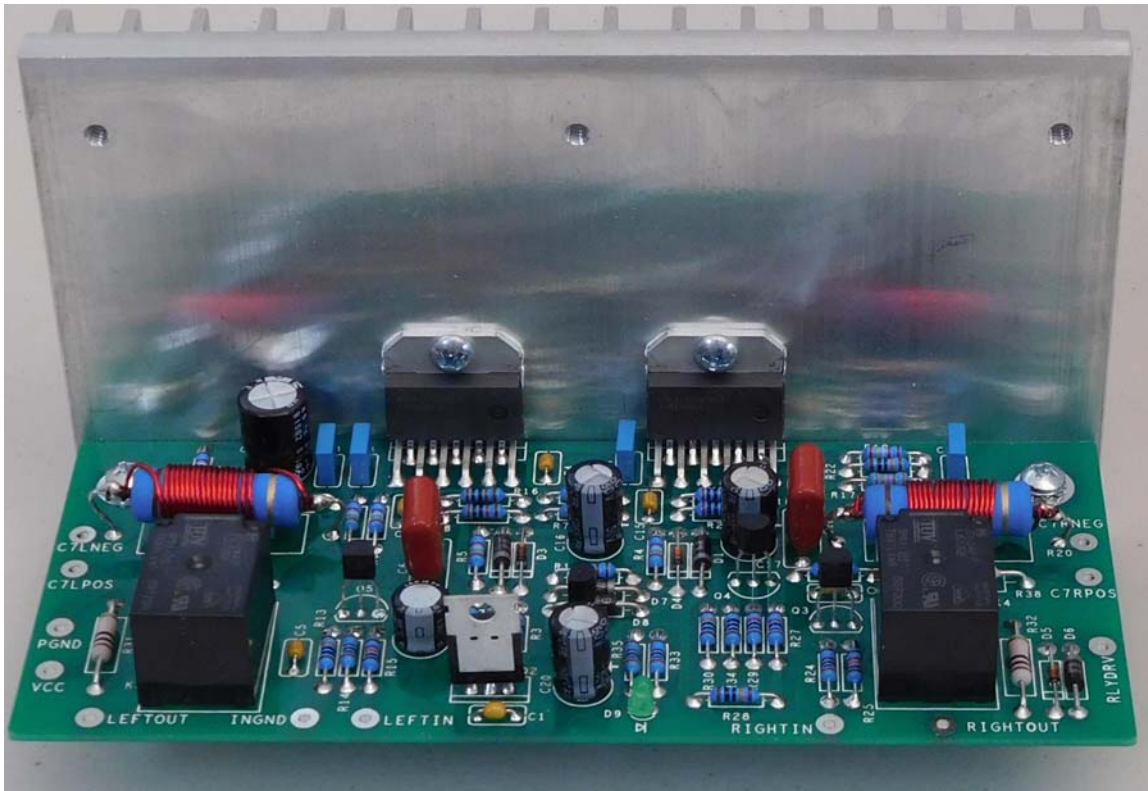
Figure 12-Assembled amplifier on main heatsink
