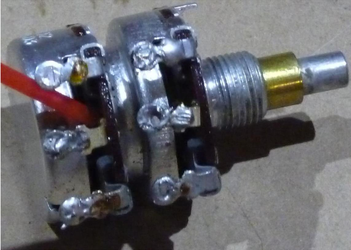
Figure 4 – Spraying contact cleaner into a control. Repeat for the section closer to the shaft.
