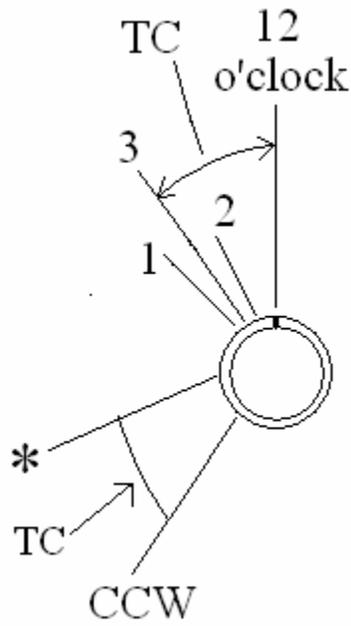
Figure 3 - \* marks the new position for the CCW extreme of the pot's travel
