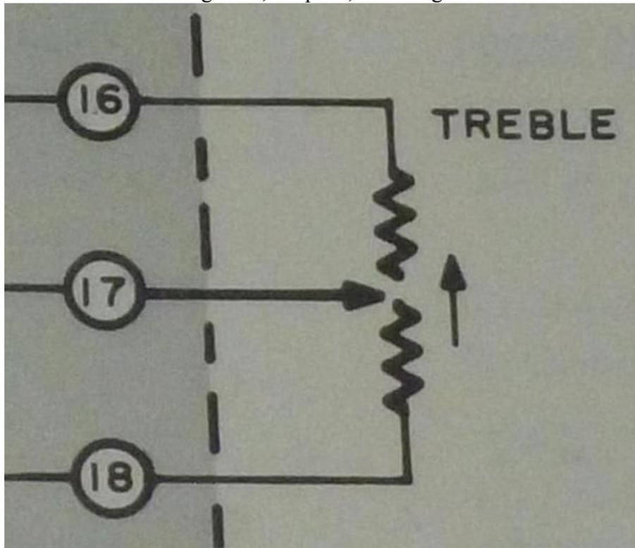
Figure 1 – close-up of the drawing of the treble pot in the PAT-4 schematic clearly shows the break in the center of the resistive element
