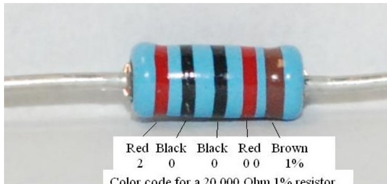
Figure 13-demonstrating the resistor color code
