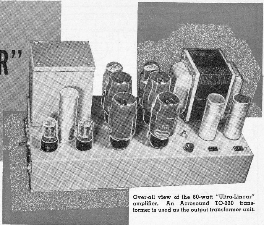
Over-all view of the 60-watt "Ultra-Linear" amplifier. An Acrosound TO-330 transformer is used as the output transformer unit.
