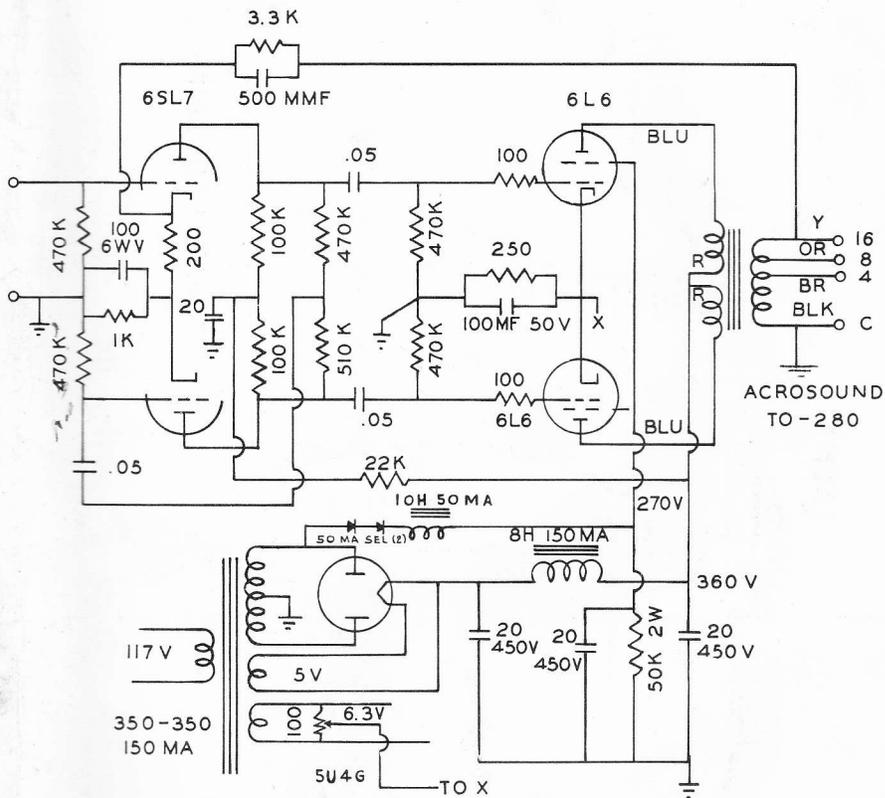
PUSH PULL PARALLEL ULTRA-LINEAR AMPLIFIER WITH TO-330 TRANSFORMER
