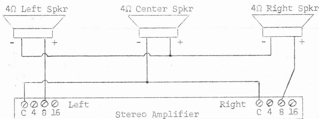
Note: 4 ohm speakers shown connect to 8 ohm amplifier taps.
