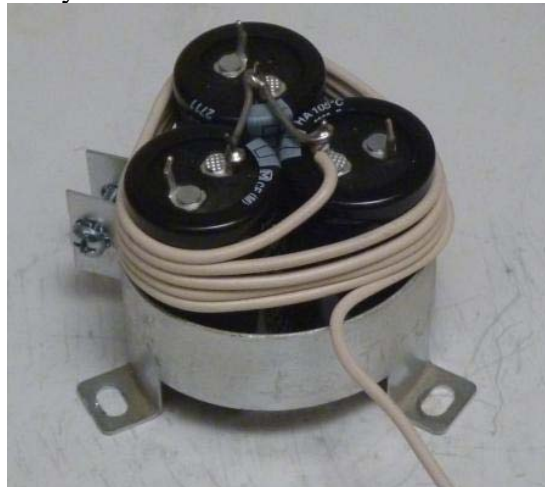
Figure 8-Inductor wound around the new C7
