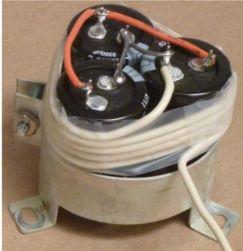
Figure 9-Adding red wires to connect positive terminals
