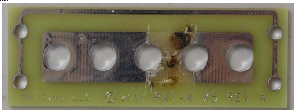
Figure 6-Copper removed from the back of the 5-RCA power to allow a split grounding arrangement
