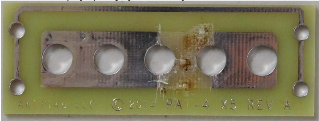
Figure 7-Cleaning up the burn marks
