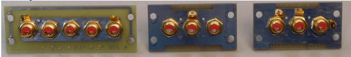
Figure 3-Jack installation, front view (right channel, red insulator jacks shown)
