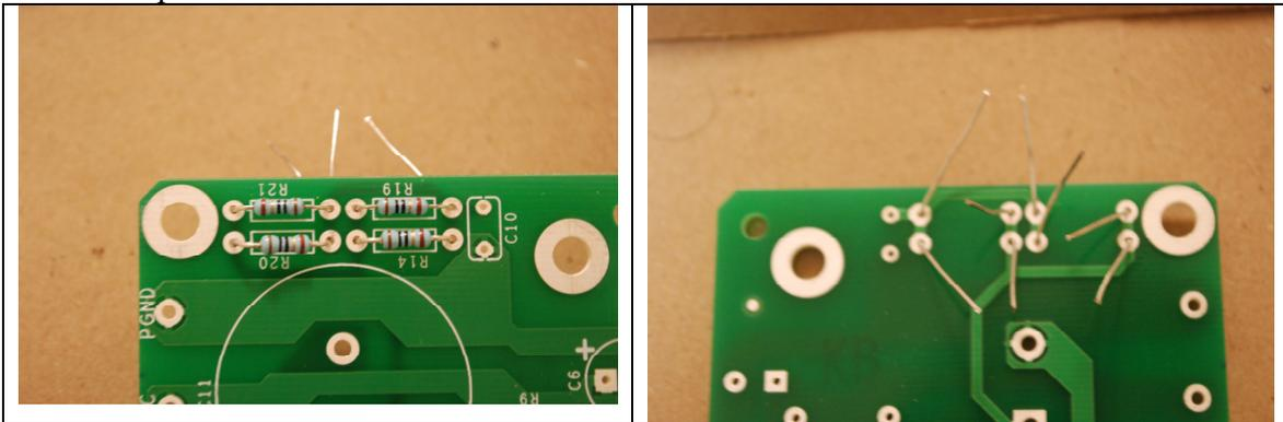
**Figure 9-**The first four resistors are installed with leads bent on the back side, but not yet soldered.
