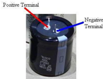
**Figure 6-Identifying the positive and negative terminals**
