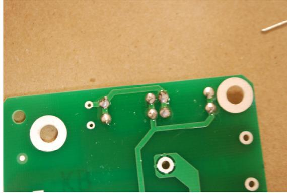
**Figure 10-leads soldered and clipped**
