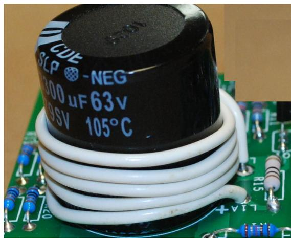
Figure 13-finishing step for the output inductor
