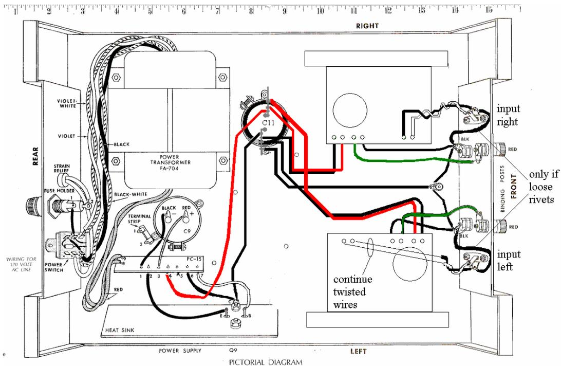
Figure 18-completed wiring
