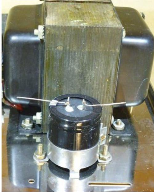
**Figure 8 - crimp and solder "antenna-like" wires to terminals of C11 to facilitate the connection of the power supply and amplifier wires**
