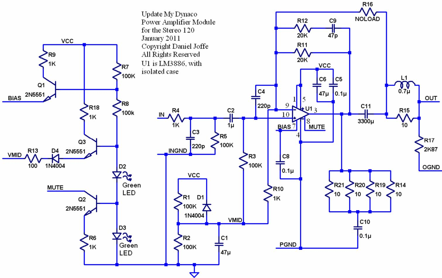
Figure 19-Schematic of amplifier module
