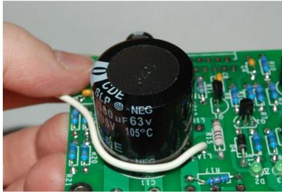
Figure 12-Starting to wind the output inductor
