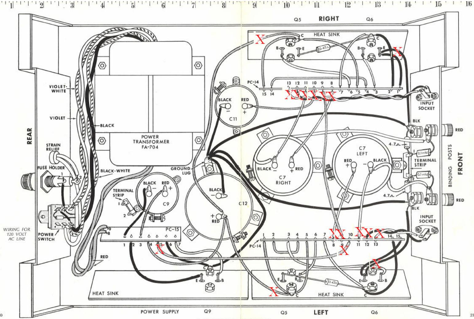
Figure 2-Location diagram for cutting wires
