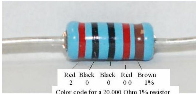
Figure 20-demonstrating the resistor color code
