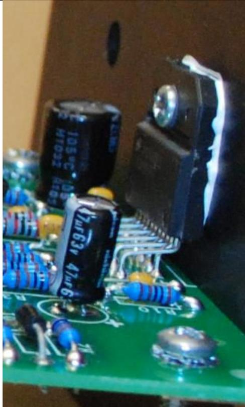
**Figure 16-**The LM3886 sits up off the board to avoid shorts between the front and back rows of pins. The body should be at right angles to the circuit board (note-detail shows original heat sink, not super heatsink, but only the LM3886 mounting height detail is of importance)
