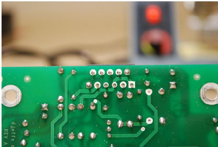
**Figure 15-LM3886 installation step three, just the corner pins are soldered**
