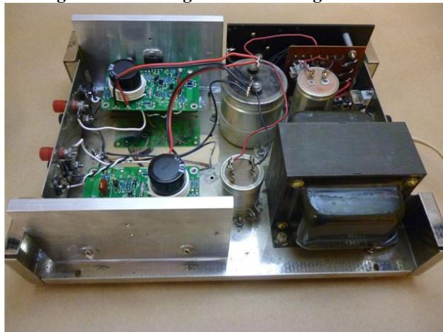
**Figure 16-Showing the Final Wiring (shown with isolated, rather than original input jacks)**
