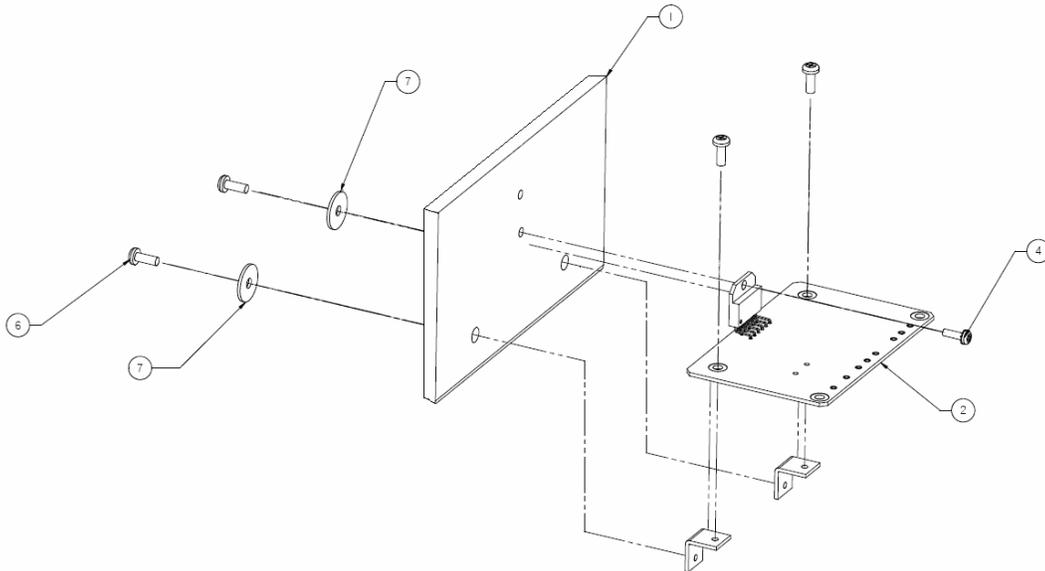
**Figure 11-Assembling the circuit board to the heat sink**
