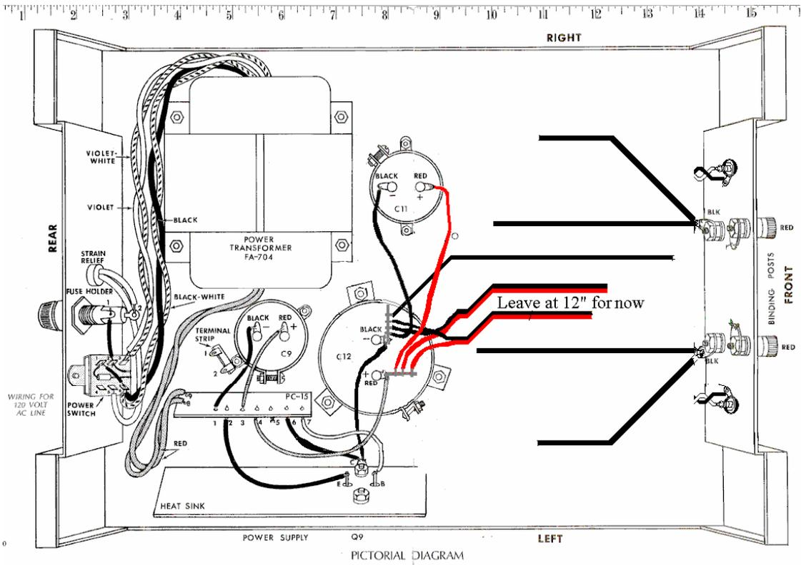
Figure 18-Rewiring the power and half the grounds
