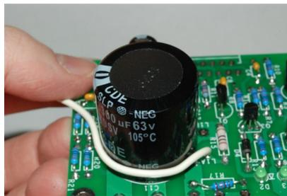
**Figure 9-Starting to wind the output inductor**
