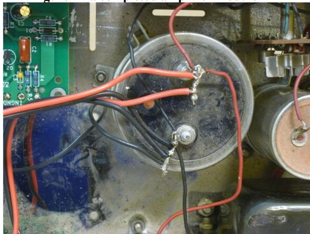
**Figure 15-Showing Detail of wiring to C12**
