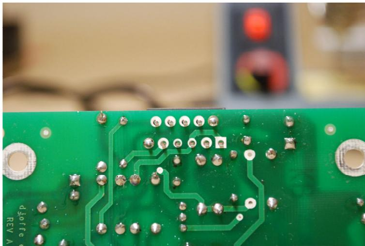
**Figure 12-LM3886 installation step three, just the corner pins are soldered**
