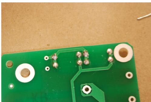
**Figure 7-leads soldered and clipped**
