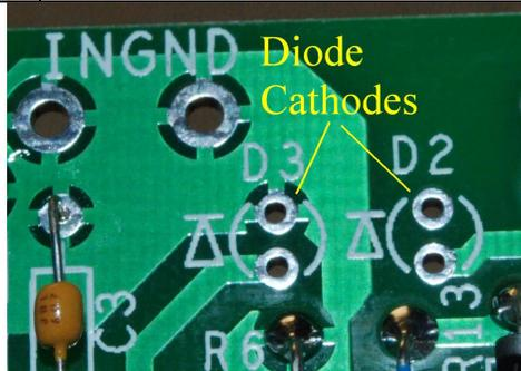
Figure 8-showing LED cathode orientation
