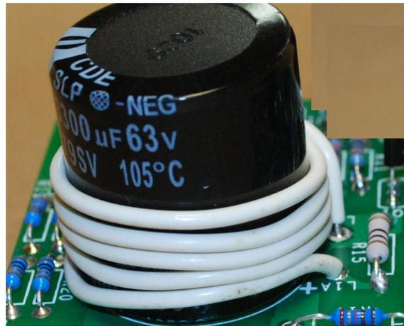
**Figure 10-finishing step for the output inductor**
