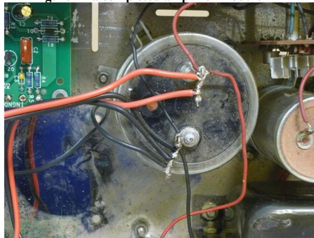
**Figure 15-Showing Detail of wiring to C12**
