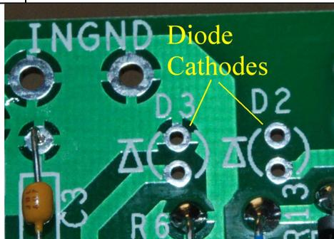
Figure 8-showing LED cathode orientation
