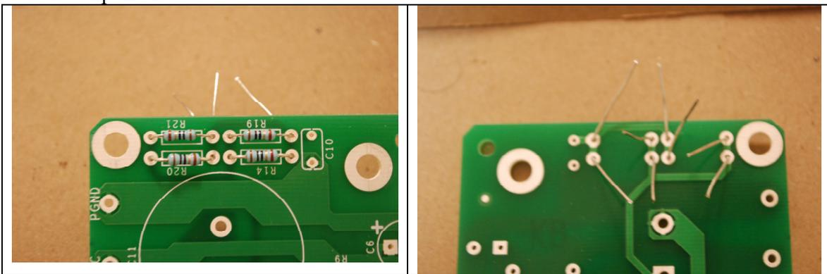
Figure 6-The first four resistors are installed with leads bent on the back side, but not yet soldered.
