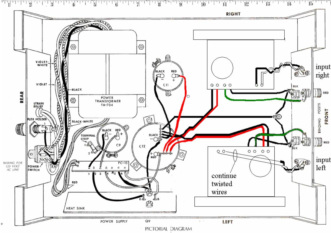
Figure 19-completed wiring
