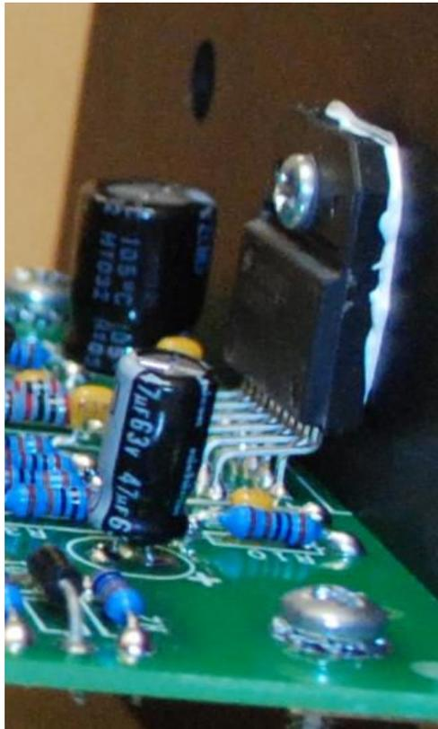
Figure 13-The LM3886 sits up off the board to avoid shorts between the front and back rows of pins.
