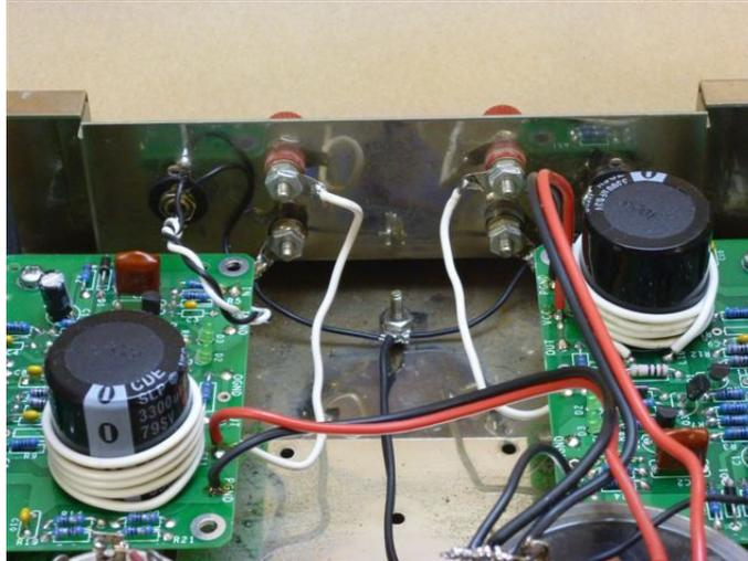
Figure 17-Final wiring, input panel detail (isolated input jacks versus standard non-isolated jacks)
