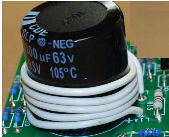
Figure 14-finishing step for the output inductor
