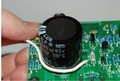
Figure 13-Starting to wind the output inductor
