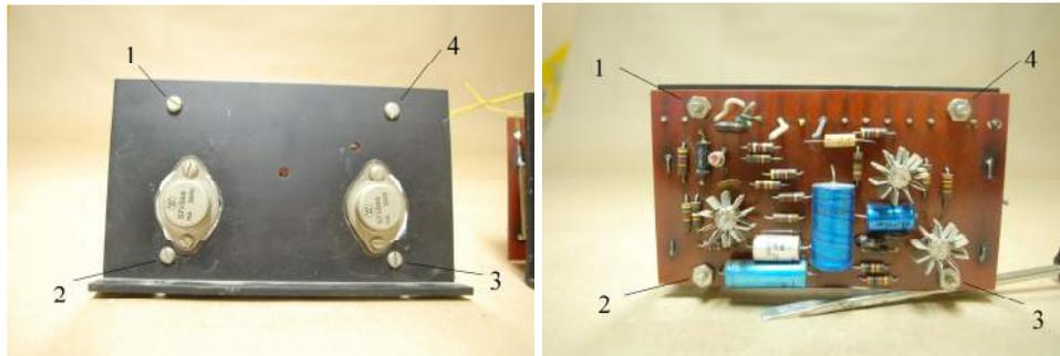
**Figure 5- Separating heat sinks and circuit boards**
