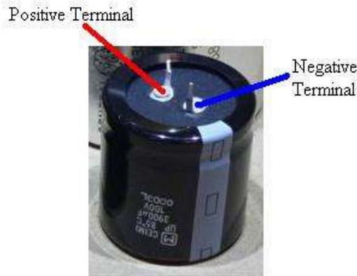
**Figure 7-Identifying the positive and negative terminals**
