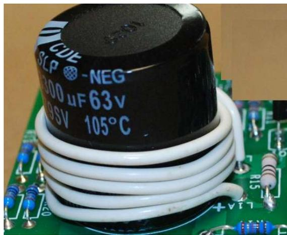
Figure 14-finishing step for the output inductor
