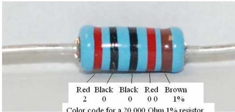
Figure 23-demonstrating the resistor color code
