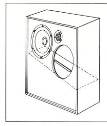
The top half of the A-50's cabinet contains the two 10" woofers and dome tweeter; the acoustic venting is between the top and bottom halves.
