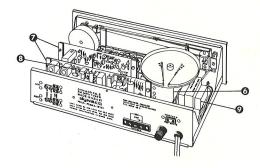
Preassembled front end supplied with kit. Preassembled etched boards for IF, multiplex, audio and power supply circuits facilitates kit construction. Seven ceramic filters and seven integrated circuits used in IF and
