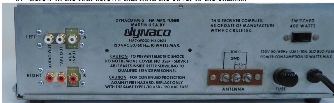
**Figure 8-New jacks installed**
