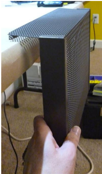
Figure 6-Gently bend the sides of the cover to make the screw holes align more easily
