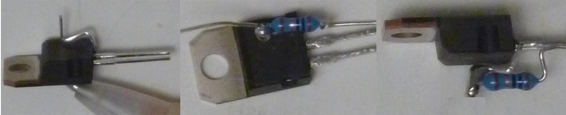
**Figure 3-Q3 with resistor added to the emitter**
