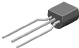
In some cases, the leads may be bent as the picture above shows. In other cases, you may have to spread the outside leads a bit to make it easier to insert them into the board.
