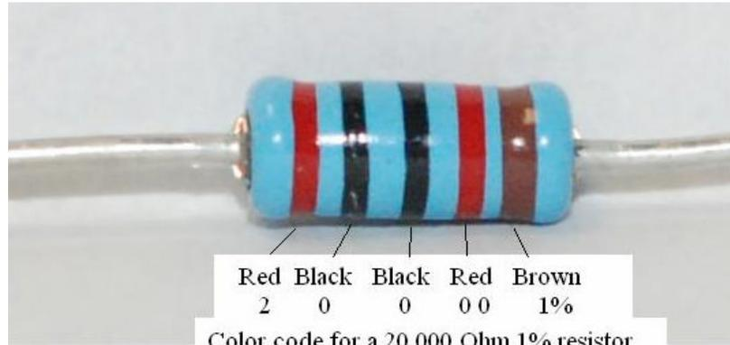
**Figure 8-demonstrating the resistor color code**
