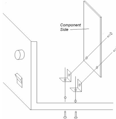
**Figure 5-Mounting the power supply to the PAT-4**
