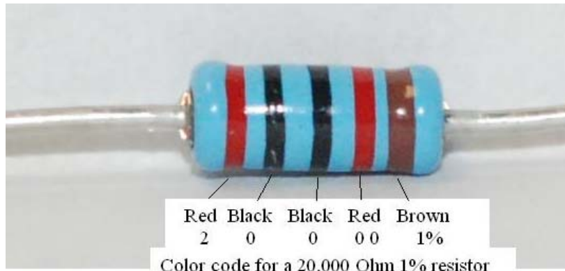
Figure 7-demonstrating the resistor color code
