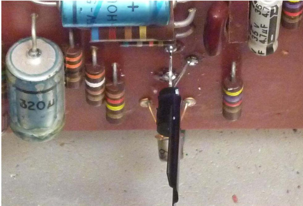
Figure 2-New transistor with heatsink installed on PCB
