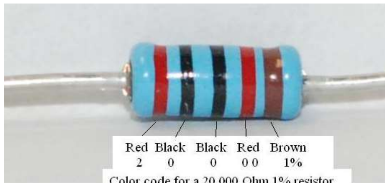
Figure 13-demonstrating the resistor color code
